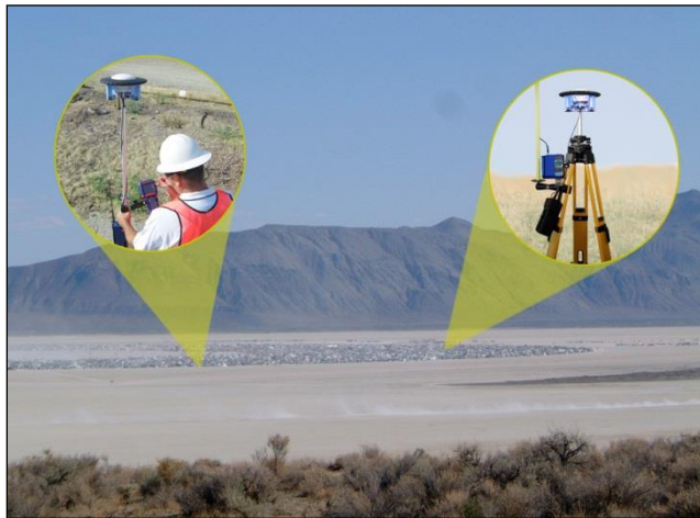
Figure 35: RTK Setup - Good Line of Sight
