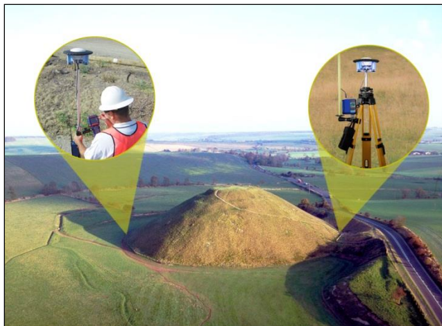
Figure 36: RTK Setup - Poor Line of Sight
